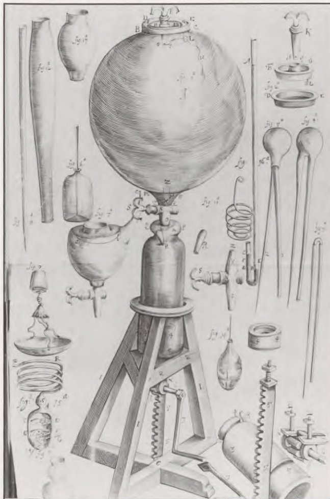
Illustration of the air pump, in Robert Boyle's New Experiments Physico-mechanical Touching the Spring of the Air , 1662. (University of Melbourne Library Collection.)
