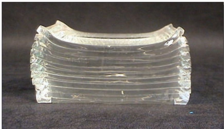
A slab of optical glass, an early attempt at producing optical glass as part of Australia's Optical Munitions Program. It was made in the Chemistry Department, University of Melbourne, c. 1941–1942, and comprises eleven glass plates, 7.0 x 13.5 x 9.5 cm, 'welded' together. (Physics Museum Collection, School of Physics, University of Melbourne, reg. no. 70)
